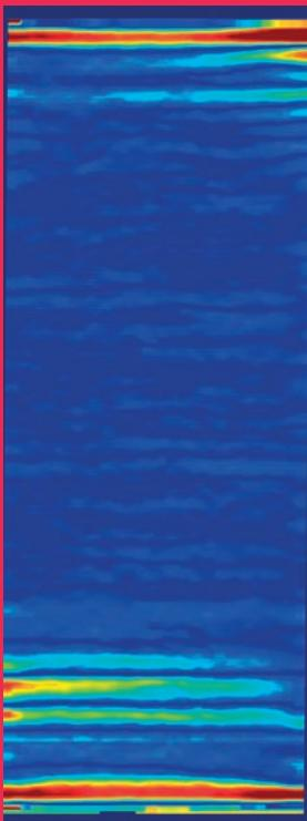
Optical distortion caused by a lack of flatness in the glass is measured by comparing the reflected image with reference patterns. The result is provided in diopters (where one diopter represents the distortion created by a curvature radius of 2 meters). The system has a resolution of 0.002 diopters.
