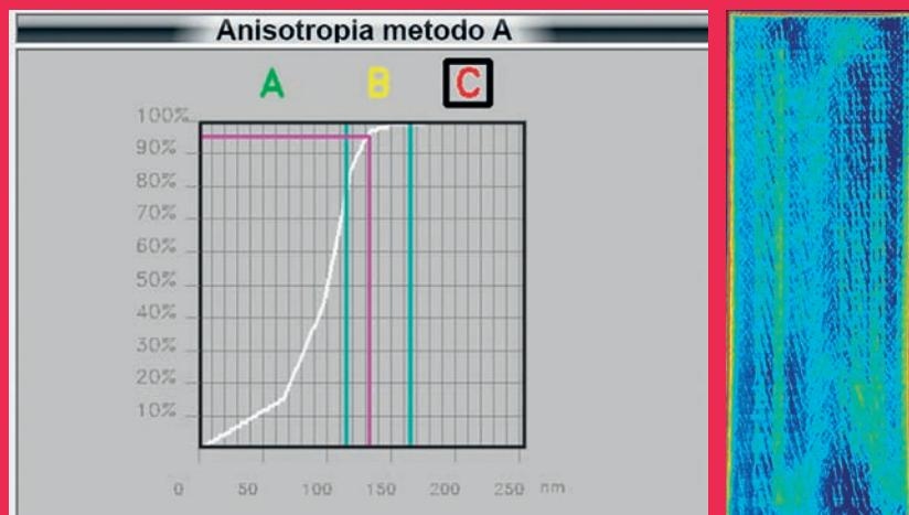
Iridescence, or the so-called "leopard spots," is caused by the anisotropy of the glass.
